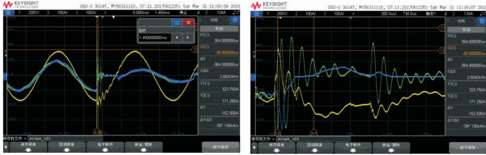
Fig\_6 Severe fluctuation of grid voltage
